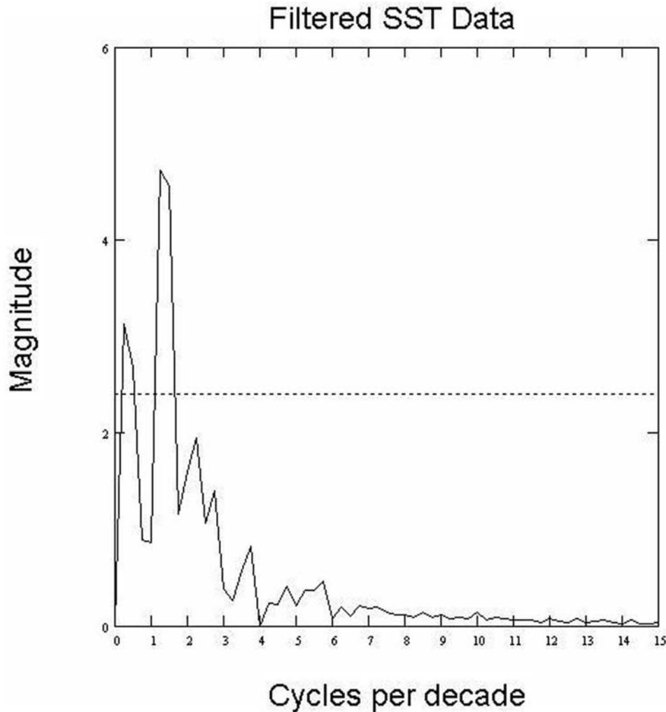
**Figure 5.** The power spectra for the filtered mean SSTs in the SSCS region. The filter was set in order to remove the signal for time periods smaller than 2 years. The abscissa is cycles per decade; thus 10 is 10 cycles per decade or the annual cycle. The dashed line represents the 99% confidence interval for accepting the red noise spectrum null hypothesis.
